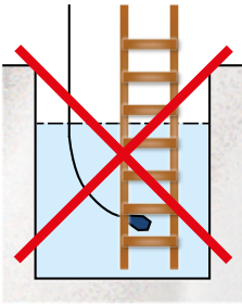
Image 4. Take care to ensure the free movement of the float.
